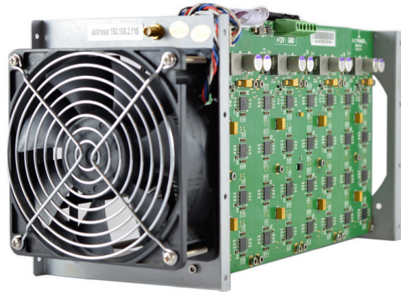
Figure 2: Left: A USB hub hosting an array of ASICMINER Block Erupter USB-stick style bitcoin miners, and a USB-powered cooling fan. Each USB-stick uses a 130-nm ASIC that hashes at 330 MH/s, or about half the performance of $450 28-nm AMD 7970 GPU. Right: Bitmain Antminer machine with two parallel sea-of-ASICs PCBs. Photo Credits: DennisD7, and dogie of bitcointalk.org.
