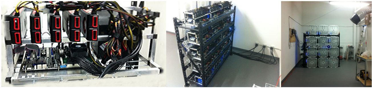
Figure 1: Left: An open-air GPU mining rig. Five GPUs are suspended above the motherboards, with riser cables connecting the GPU’s PCI-E connector to the motherboard below, and a single high-wattage power supply. Center, Right: Two pictures of a homebrew 69-GPU Bitcoin mining datacenter. Note the ample power cabling, left, and the cooling system, consisting of box fans and an air duct, right. Photos Credit: James Gibson (gigavps).
