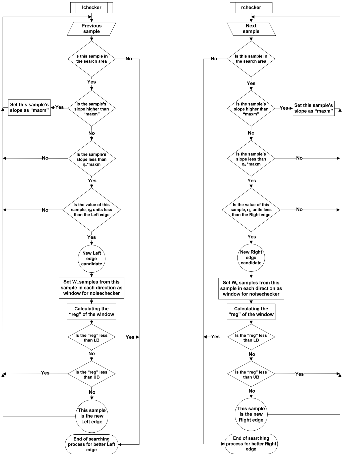
Figure 3-c. General flow-chart of the HSEDF code describing the structure of the proposed detection-delineation algorithm. Correction of primitive identified QRS onset-offset locations via checking the level of noise of the primer point via lchecker and rchecker functions (Second major operation).
